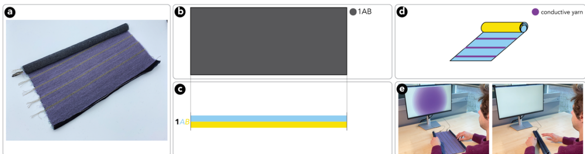
Fig. 4 – a) The Rollable Textile-form Interface is designed to curl into a tube. It consists of a single-layer compound weave structure with two unbalanced weft sets. b) The MoB shows with one colour that the same binding is applied to the entire sample. One weave structure is weft-facing (faces up), and the other is warp-facing (faces down). With the unbalanced weaves and using yarns with different stiffness, one side of the fabric tends to curl along the warp direction when released from the loom. c) Layer relationship: Warp 1 weaves weft A on top and weft B at the bottom. d) Placement of the conductive yarn. e) Interaction with the textile-form interface.
